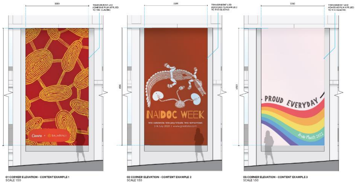
Figure 45: Examples provided during assessment of content proposed to be displayed within corner glazing signage (LED glazing film).
