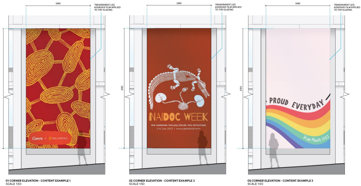
Figure 33: Example content to be displayed within corner signage, LED adhesive film applied to glazing.
