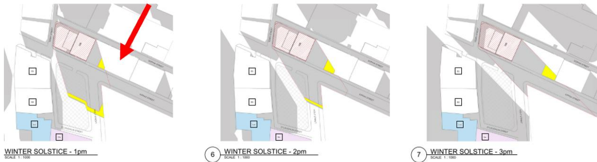
Figure 51: shadow impacts for the roof area of 26-44 Kippax Street (red arrow, yellow shading), at the winter solstice.
